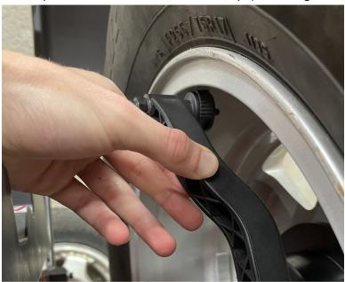
• Without returning the distance arm to the home position, immediately place the distance arm to your desired outside tape weight location, hold the arm in place and the machine will beep (see image below)
