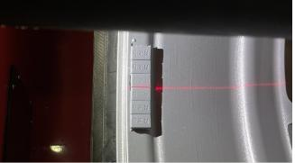
Rotate the wheel to the outer position shown on the display. The machine's laser will turn on and you will add the weight at 6 o'clock to the outside of the wheel. In this case, the weight called for is 1.00 oz, so we placed 0.50 oz on each side of the laser (see images below).
