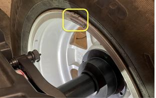
• Rotate the wheel to the outer position shown on the display. The machine's laser will turn on and you will add the weight at 6 o'clock to the outside of the wheel. In this case, the weight called for is 1.00 oz, so we placed 0.50 oz on each side of the laser (see images below).
