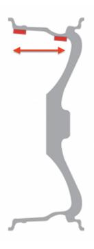
If the distance between your tape weights is less than 4" or 5", this could cause an inaccurate balance. The weights should be greater than 4" or 5" apart.
