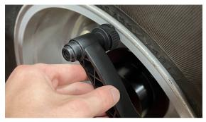
• Without returning the distance arm to the home position, immediately place the distance arm to your desired outside tape weight location, hold the arm in place and the machine will beep (see image below)
