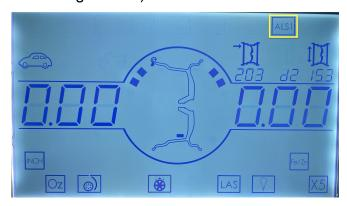
Place the distance arm against the bead of the wheel, hold the arm in place and the machine will beep (see image below)
