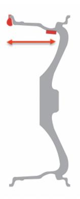
If the distance between your weights is less than 4" or 5", this could cause an inaccurate balance. The weights should be greater than 4" or 5" apart.
