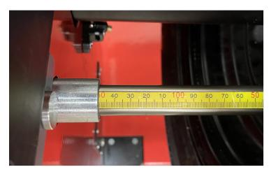
At the home screen, change DIA +/- and DIS +/- to numbers that are different than the wheels actual parameters
