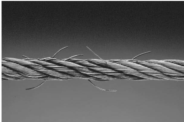
Cable With Broken Wires
