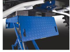
**Load bearing hinged ramps** with polymer rollers allow additional access to perform wheel / brake work. The ramps fold up, lock in place and increase lifting capabilities by extending the pick-up point surface area. Hinged ramps fold 65 degrees down and away, allowing for more access to service vehicle.
