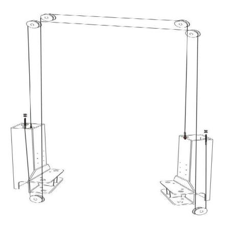
Key points for assembly: the two steel cables shall be adjusted to equal tension in order to verify the
