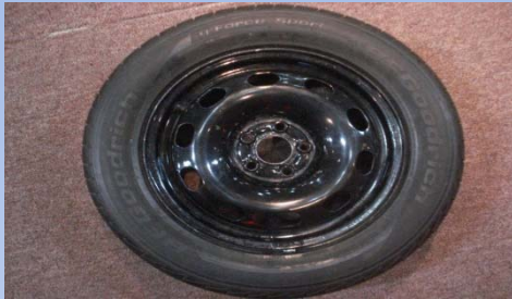
15" Diameter, 6" wide steel wheel assembly
