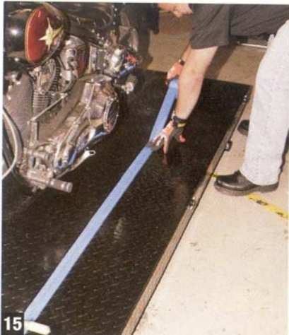
15 James ran some tape down the seam where the lift and extension met, so that no bolts would fall through and get lost. Then, he connected the air supply to the foot pedal and lifted the bike so we could start to remove the transmission.
